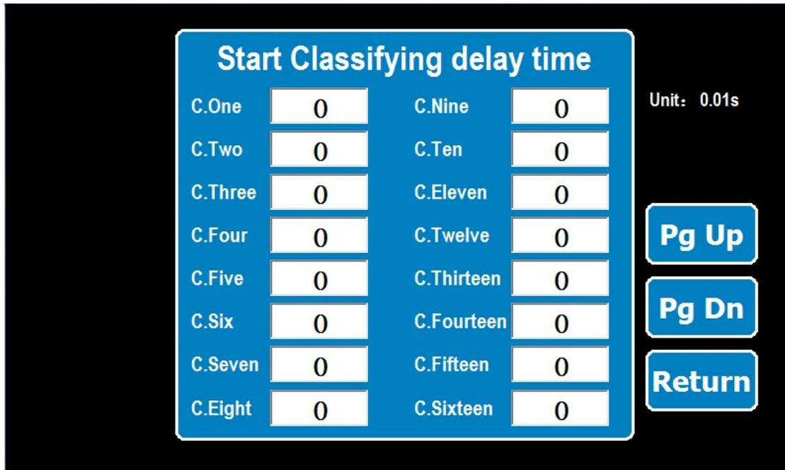
This interface can set the delay time of the dialing board. The customers can set this time in their own factory. Click “Pg Dn”.
